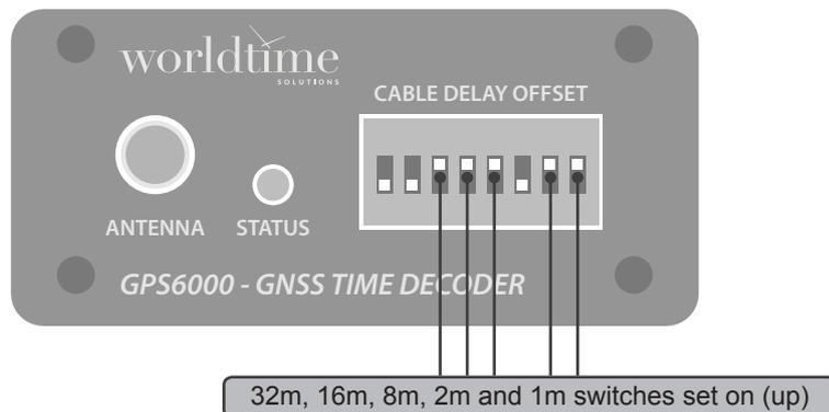
Figure 2.6 - Example 59m cable delay offset
