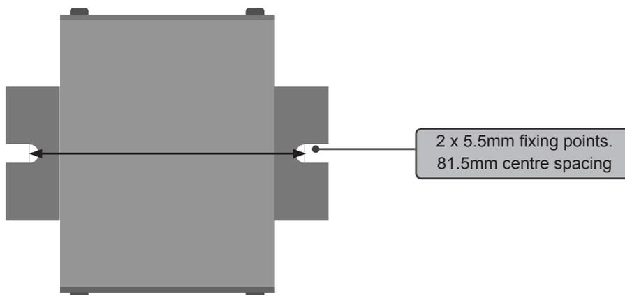
Figure 2.1 - GNSS decoder enclosure mounting dimensions
