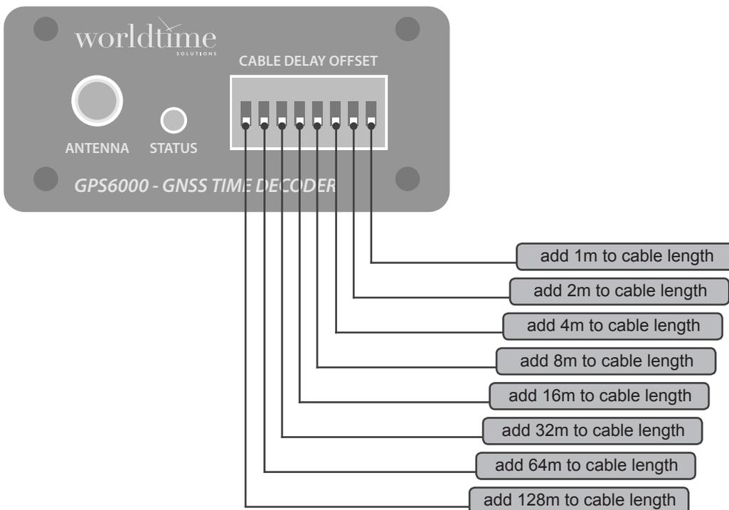
Figure 2.4 - The cable delay offset switch bank
