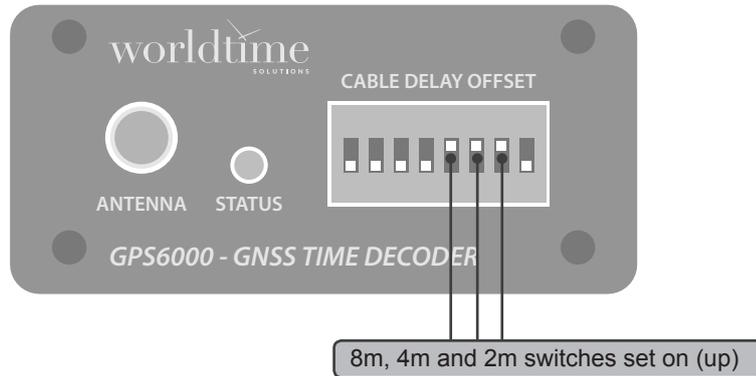
Figure 2.5 - Example 14m cable delay offset
